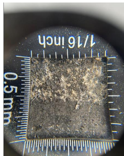
Roof Tiles – showing weathering and exposure of asbestos fibres
